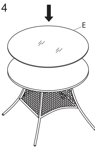
Remark: Be noted, during assembly, we recommend only to tighten all screws with 80% fastening, when having all screws in correct position, and tightened to 80% - then OK to tighten to 100%, to avoid any distortion, bendings.
