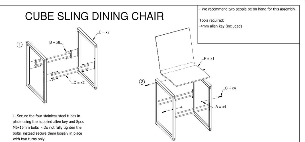
2a. Line the seat/back assembly up with the 4 upper holes in the teak frames and secure them loosely in place (two turns only) with the custom bolt M8x50mm - Note that there must be Ø12x7mm spacers between the teak frames and the seat assembly
